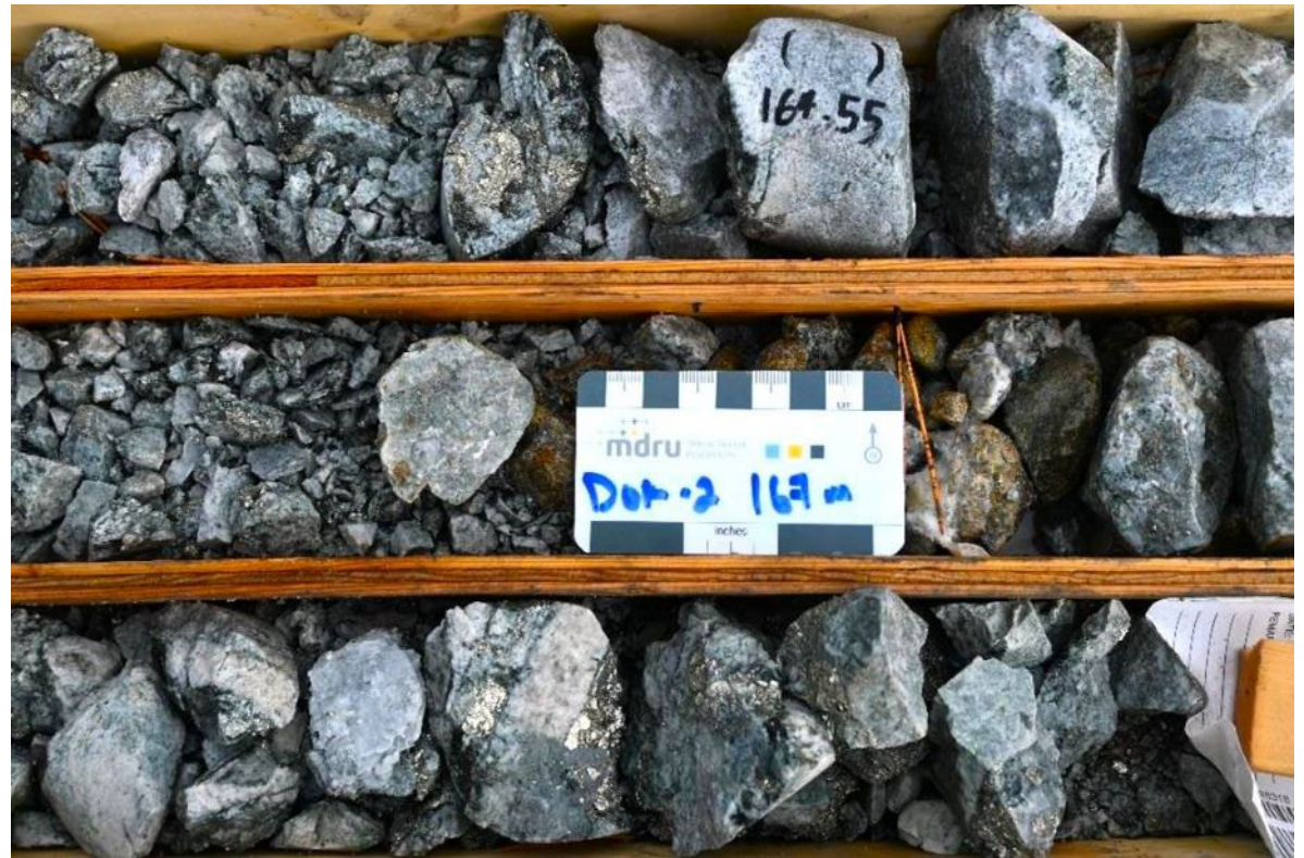
Sample from DK2023-002 showing a zone of intense sulphide stockwork. 164.55 is a Terraspec (SWIR) sample location.
